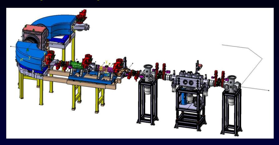
Double Valves makes it longer working on shortening the cooler module Present length ~4 m
